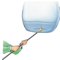
Use a long-handled knife to cut the bag.
