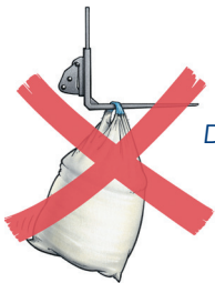
Bulk bags should be lifted with a lifting hook
